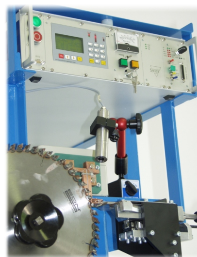
detail view of induction brazing equipment with optional temperature control THERMCON
